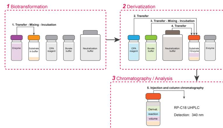
**Figure 1:** Pipetting scheme for the biotransformation and analysis of the glutaminase assay in the autosampler vials.
